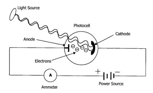
The cell has two metal electrodes sealed in an evacuated tube. The air has been removed to keep the metal surface clean and to keep electrons from being stopped by the air molecules. The large electrode, the cathode, is usually coated with cesium or some other alkali metal. The second electrode, the anode, is made of a thin wire so it does not block any radiation. The tube is often made of quartz to permit ultraviolet wavelengths to pass through.
